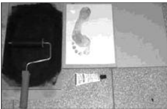
FIGURE 1: The footprint system composed of Sirchie fingerprint ink, special roller, smooth thick glass and a piece of paper.
