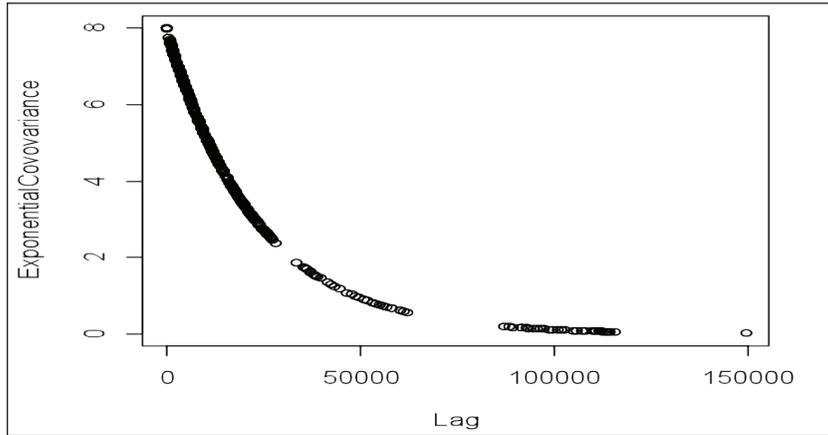
FIGURE 2(a): Exponential covariogram oil and gas pipeline data.
