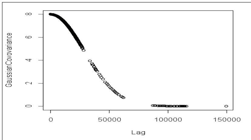
FIGURE 2(c): Gaussian covariogram oil and gas pipeline data.
