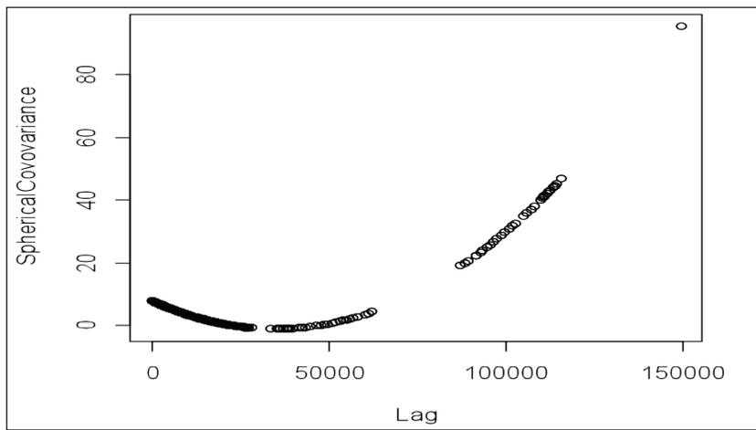
FIGURE 2(b): Spherical covariogram oil and gas pipeline data.
