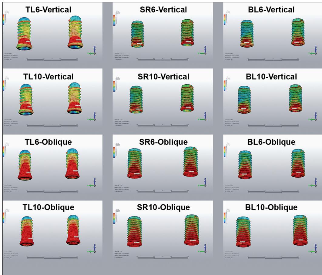
FIGURE 3: von Mises stresses in implant models. TL6: Tissue-level and non-engaging titanium base abutment with 6 mm crown height; TL10: Tissue-level and non-engaging titanium base abutment with 10 mm crown height; SR6: Bone-level and screw-retained abutment with 6 mm crown height; SR10: Bone-level and screw-retained abutment with 10 mm crown height; BL6: Bone-level and non-engaging titanium base abutment with 6 mm crown height; BL10: Bone-level and non-engaging titanium base abutment with 10 mm crown height.
