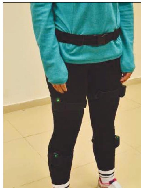
FIGURE 3: Sensors for 3D gait-analysis.
