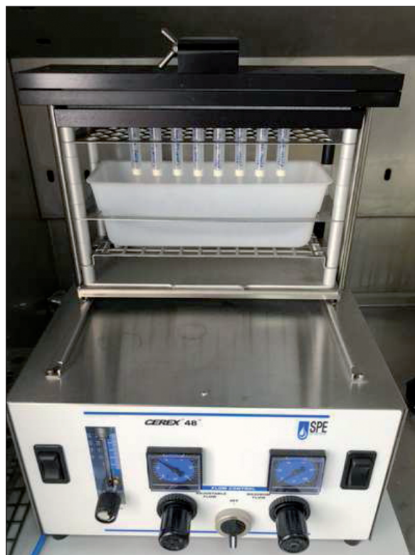
FIGURE 2: The view of SPE set-up with Positive Pressure Manifold (PPM).
