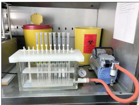
FIGURE 1: The view of SPE set-up with Negative Pressure Manifold (NPM).
