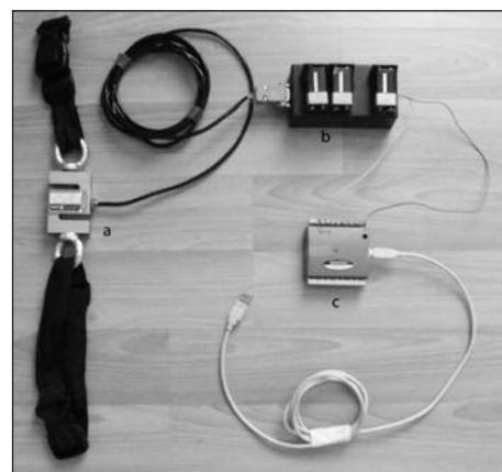
FIGURE 1: Force transducer; a: loadcell and its mounting kit, b: amplifier, c: DAQ card.
