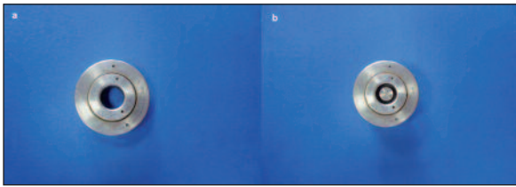
FIGURE 2: a. Stainless steel template; b. The template positioned on a stainless steel die.
