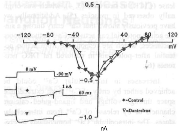
**Figure 1.** The voltage-dependent effect of dantrolene (10 μM) on the peak amplitude of calcium currents of rat DRG neurones.
