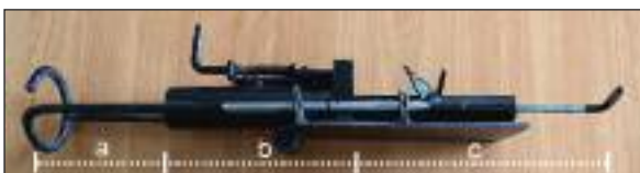
FIGURE 4: Design of a typical mole gun. (a) A metal ring in front of the gun, connected to the trigger mechanism; (b) Barrel, and (c) Trigger mechanism.
