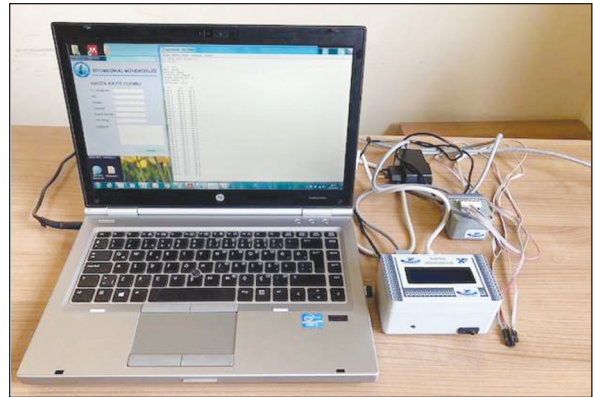
FIGURE 1: Digital heat measurement device, comprising 3 heat-sensitive sensors, a digital temperature indicator and computer software.
