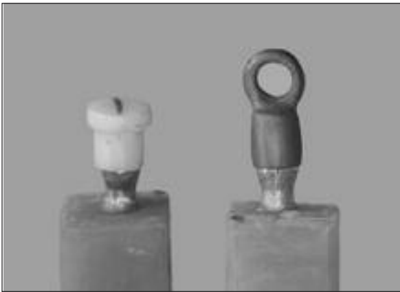
FIGURE 1: The view of Y-TZP copy-milled coping and base metal coping.
