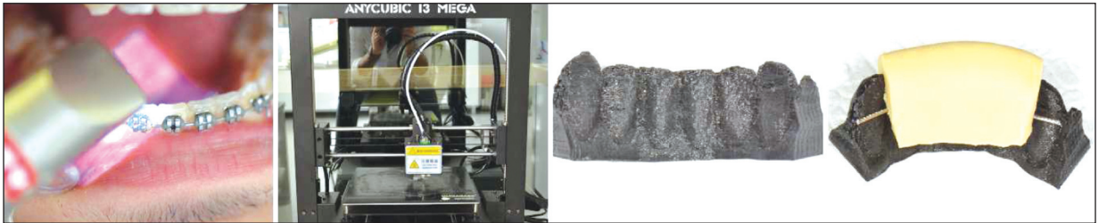
FIGURE 2: Steps of the digital method: a) intraoral scanning with CEREC b) 3D model preparation with Tinker CAD online software c) 3D printed model d) indirect retainer wire.
