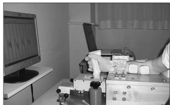
FIGURE 3: Localization of surface EMG electrodes for EMGrms records.
