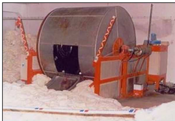
Figure 4. The softening drum (opened).
