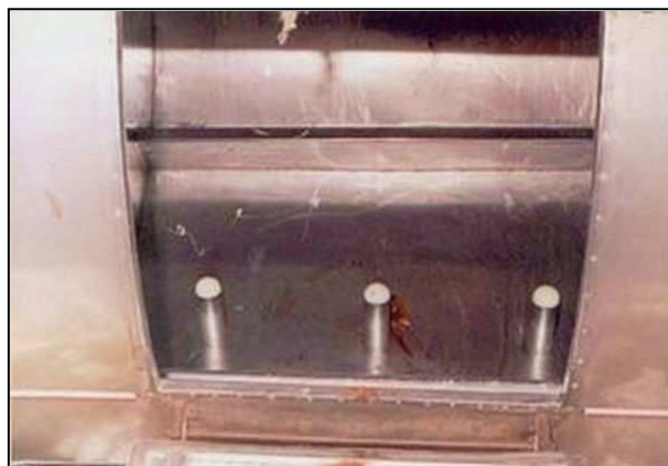
Figure 5. The interior of the softening drum (through the lid).
