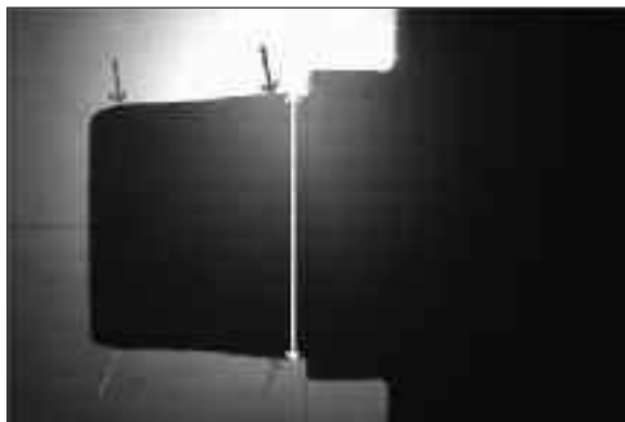
FIGURE 4: Red arrows: Deformations in occlusal, axial and neck regions. White arrow: Measurement of marginal diameter.
