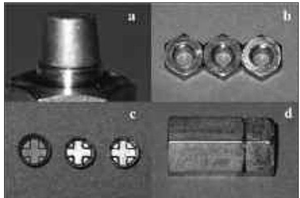
FIGURE 2: a: Placed specimen on own metal die. b: Three special stainless steel indexes. c: 3 metal frameworks with 0.2 mm, 0.3 mm and 0.4 mm thickness. d: Placed index on a metal die.
